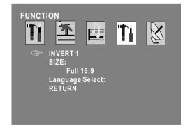
When the \*\*P symbol at "INVERT1" and Press the MENU (1) button repeatedly to invert the picture, each time the button press the picture rotate as clockwise as the diagram show.
